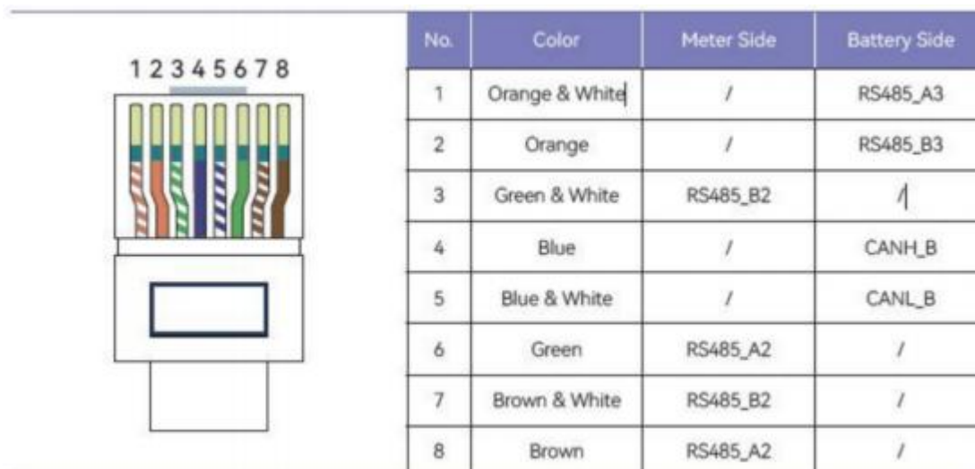
Figure 4.6-1 PCS Communication terminal definition diagram
